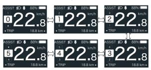
**Note:** if the controller has Boost function, can be selected this level with briefly press 2.
